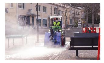
The KPL High Pressure Street Washing Unit can be used for disinfection applications. The unit is perfect for disinfecting marketplaces for example. The unit is made from materials that can handle most common disinfectants.
