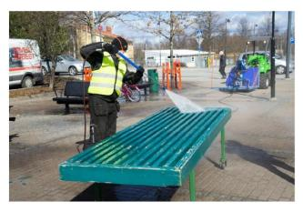
The flow of the power washer of the unit can be adjusted by adjusting the hydraulic oil flow of the pump. Another option is to swap the nozzle of the washing gun. This makes the power washing pistol a perfect disinfection tool. The same tricks work for the unit's washing boom also.
